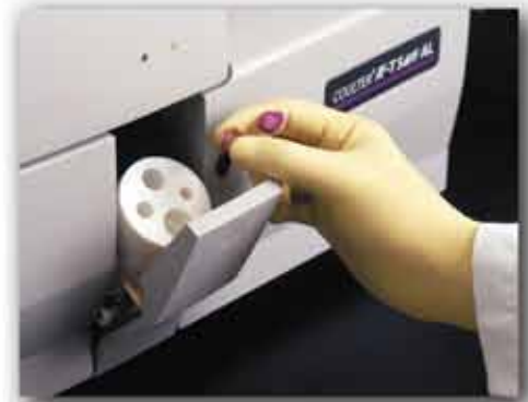
Two additional tube holders accommodate tubes of varying sizes.
