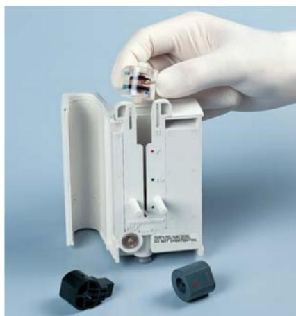
The maintenance-free electrodes are easily accessible and can be replaced in a snap.
